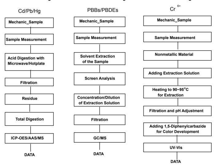
The samples were dissolved totally by pre-conditioning method according to above flow chart for Cd,Pb,Hg. Section Chief: Sharpless Park
