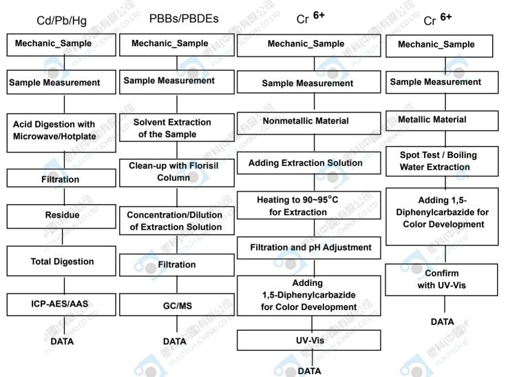
The samples were dissolved totally by pre-conditioning method according to above flow chart for Cd,Pb,Hg. Section Chief: Shapless Park
